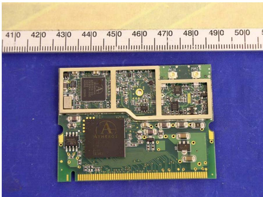
**EUT – Transceiver Solder View with Shielding**
