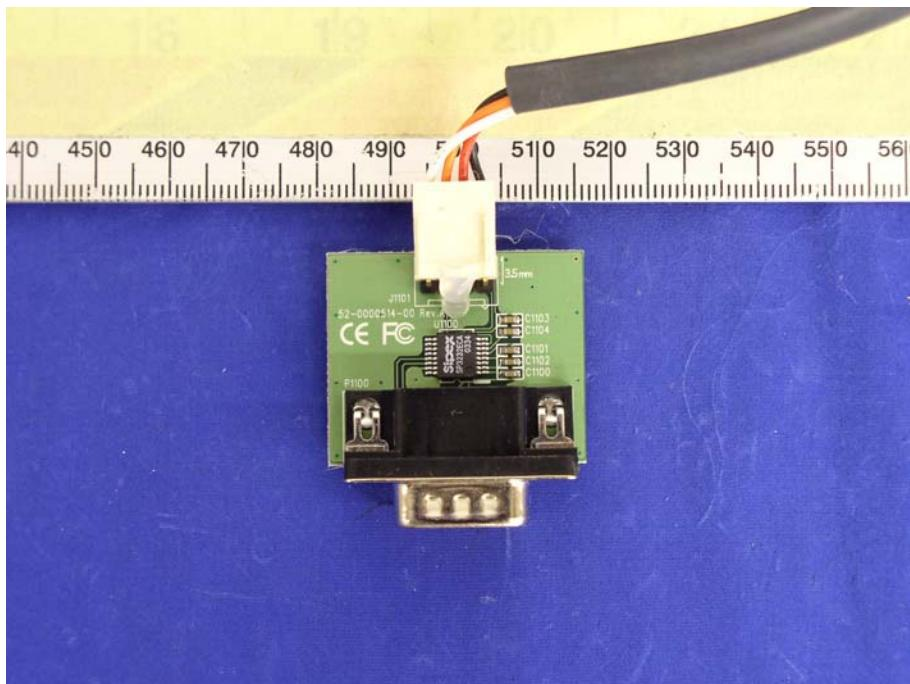
**EUT – Transceiver Component View with Shielding**
