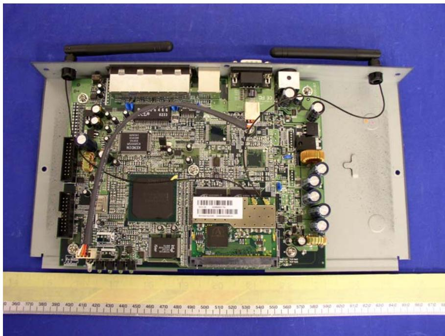
**EUT – Component View with Transceiver**
