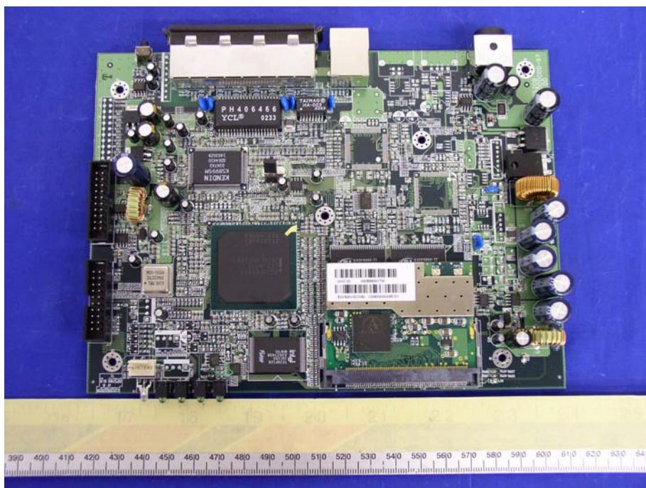
**EUT – Component View without Transceiver**
