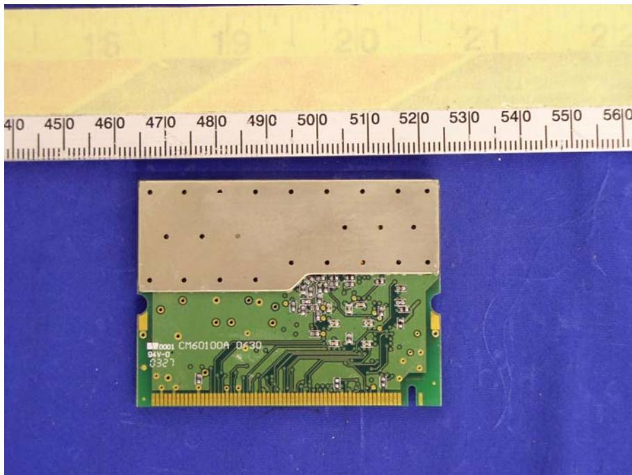
**EUT – Transceiver Solder View without Shielding**
