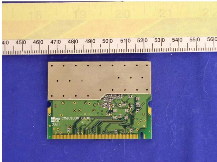
**EUT – Transceiver Solder View without Shielding**
