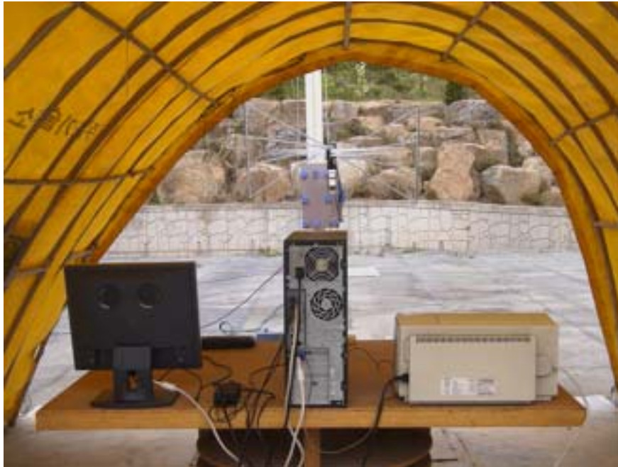
Photograph 1 : Setup for radiated Emissions
