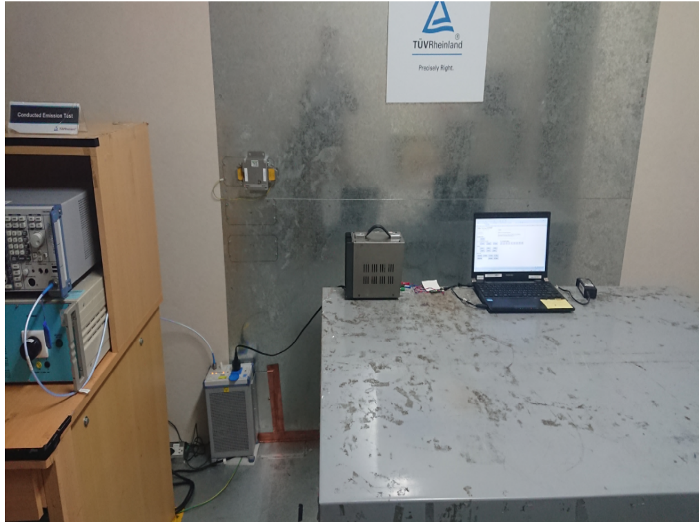
Photograph 8: Set-up for Mains Conducted testing (Back View)
