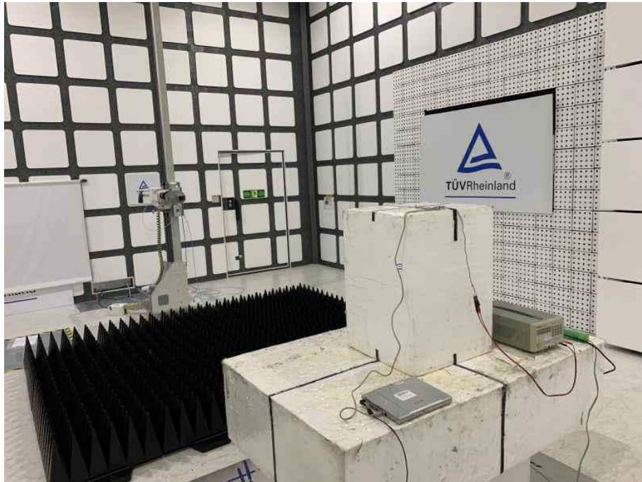
Photograph 6: Set-up for Spurious Emissions (Back View 4)
