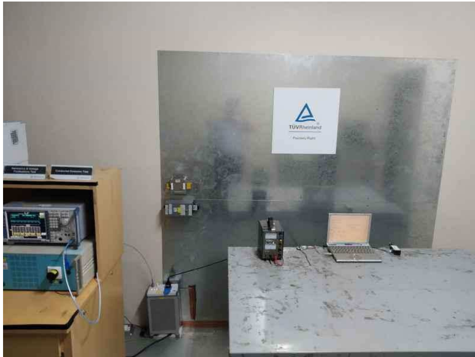
Photograph 10: Set-up for Mains Conducted testing (Back View)
