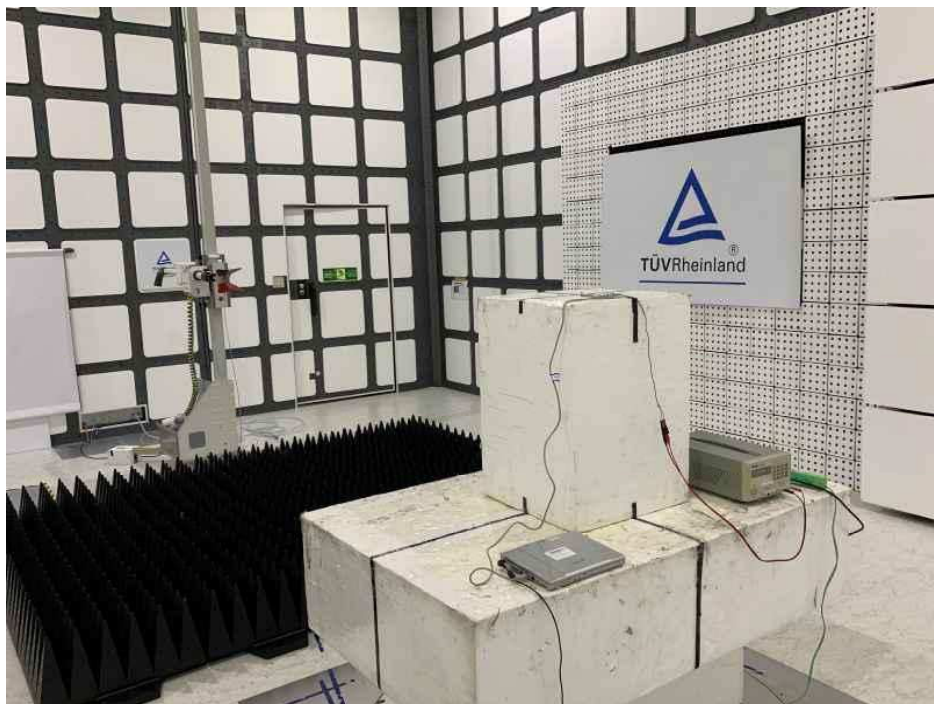
Photograph 4: Set-up for Spurious Emissions (Back View 2)
