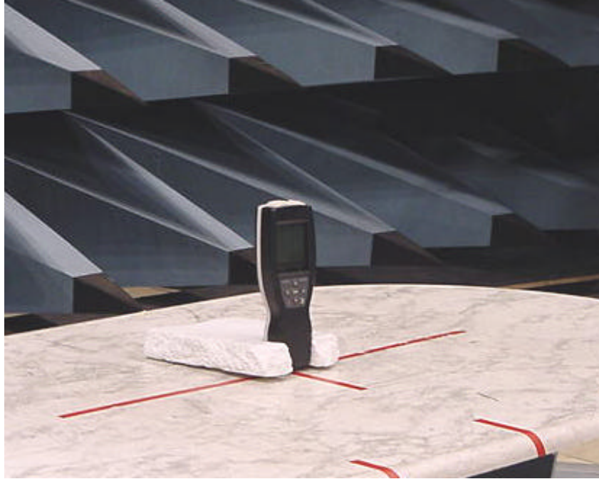
Instrument unit, radiated spurious emission 30 - 1000 MHz
