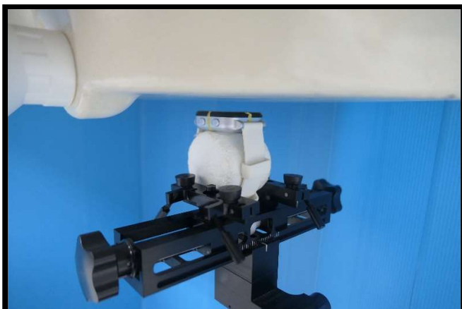
Front Face of EUT Tested at 10 mm
