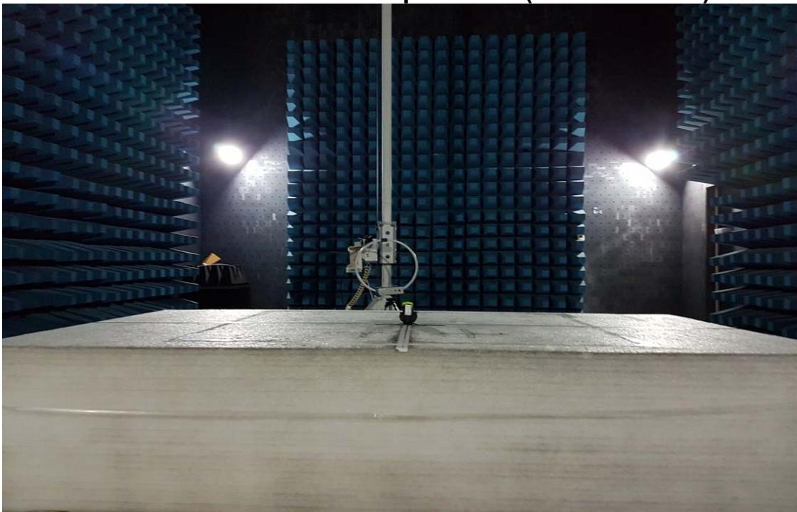
**Radiated Emission Set up Photos (Below 1GHz)**
