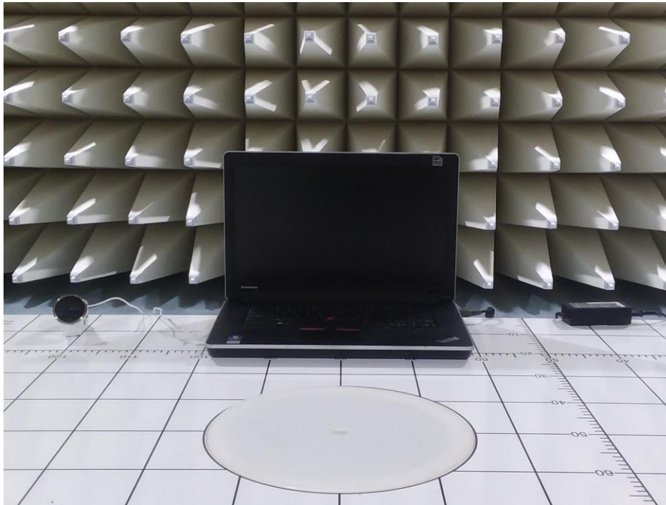
Figure B4: Radiated Emission set up
