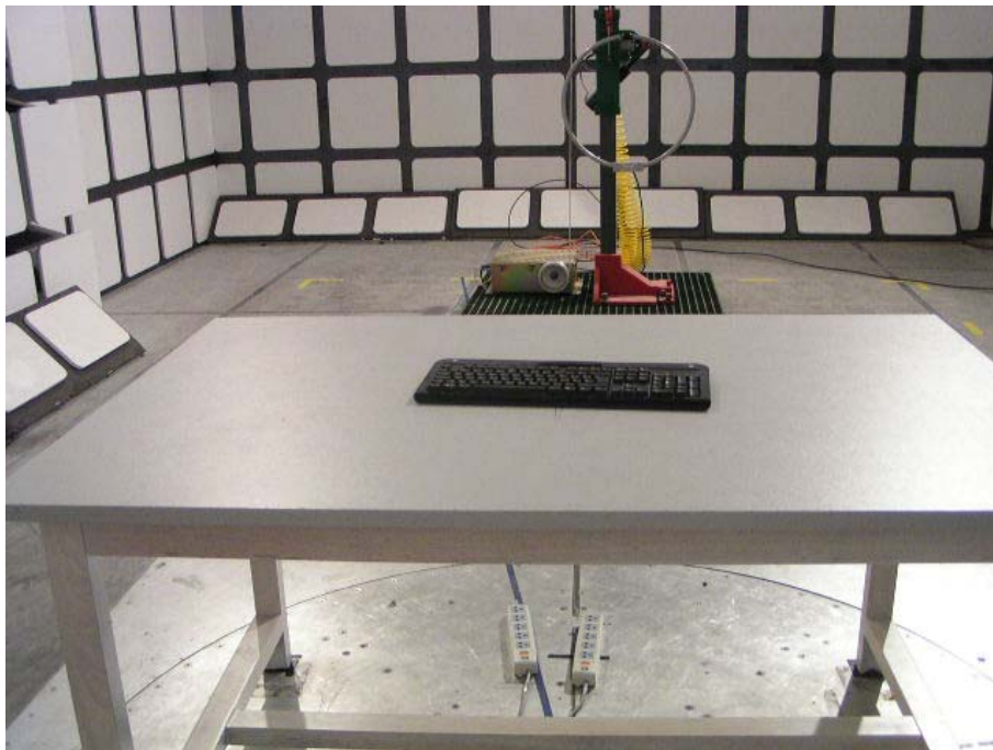
Radiated Emissions-Front View (Below 30 MHz)
