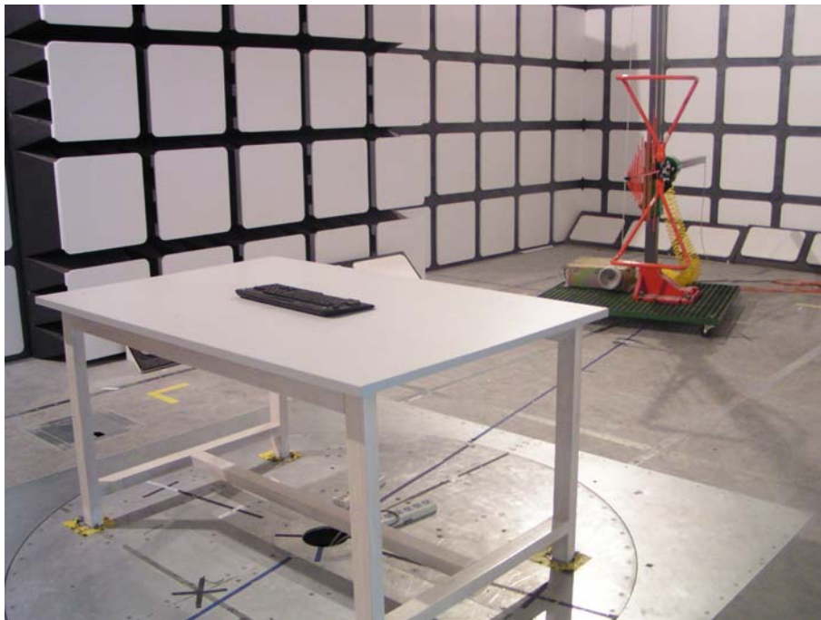
Radiated Emissions-Front View (Above 30 MHz)
