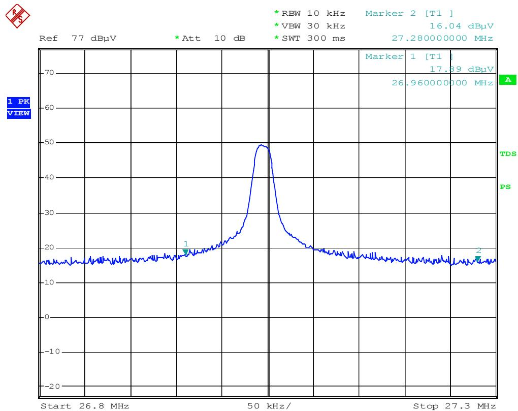
Dyna Point Wireless Optical Mouse H1FD5001 Out of Band Emission
