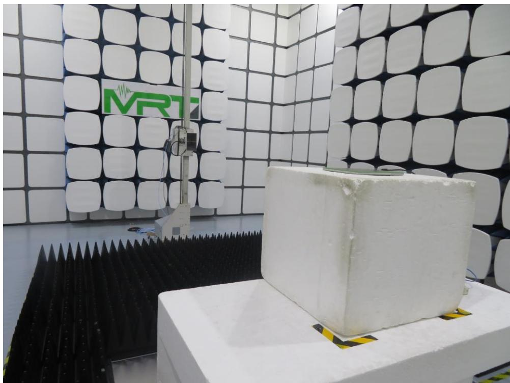
Description: Radiated Emission Test Setup for 5GHz Band-edge
