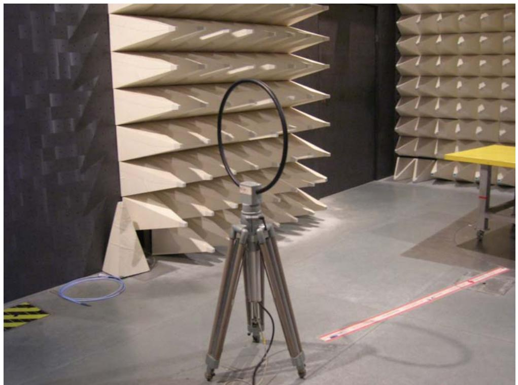
For radiated emissions 30MHz~1GHz
