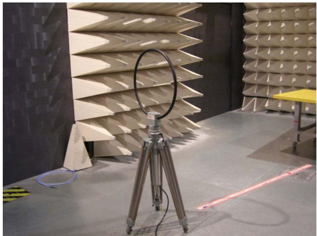
For radiated emissions 30MHz~1GHz
