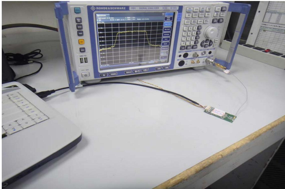
**RADIATED EMISSION SET UP PHOTOS****For printed Antenna****Below 1GHz**
