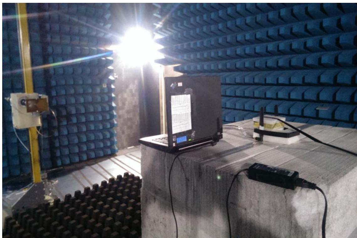
**POWERLINE CONDUCTED EMISSIONS SETUP PHOTOS****For printed Antenna**
