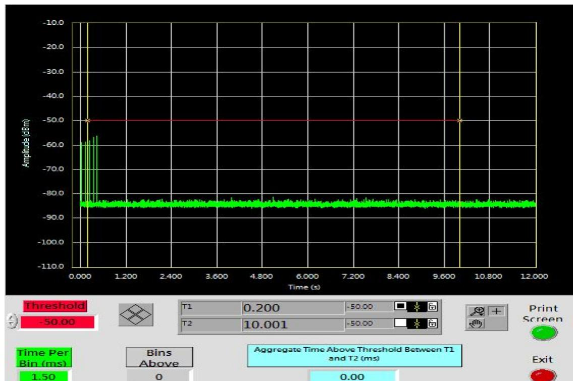
**IEEE 802.11 ac VHT 80 MHz Channel mode****Type 1 Channel Move Time Results***No non-compliance noted.*
