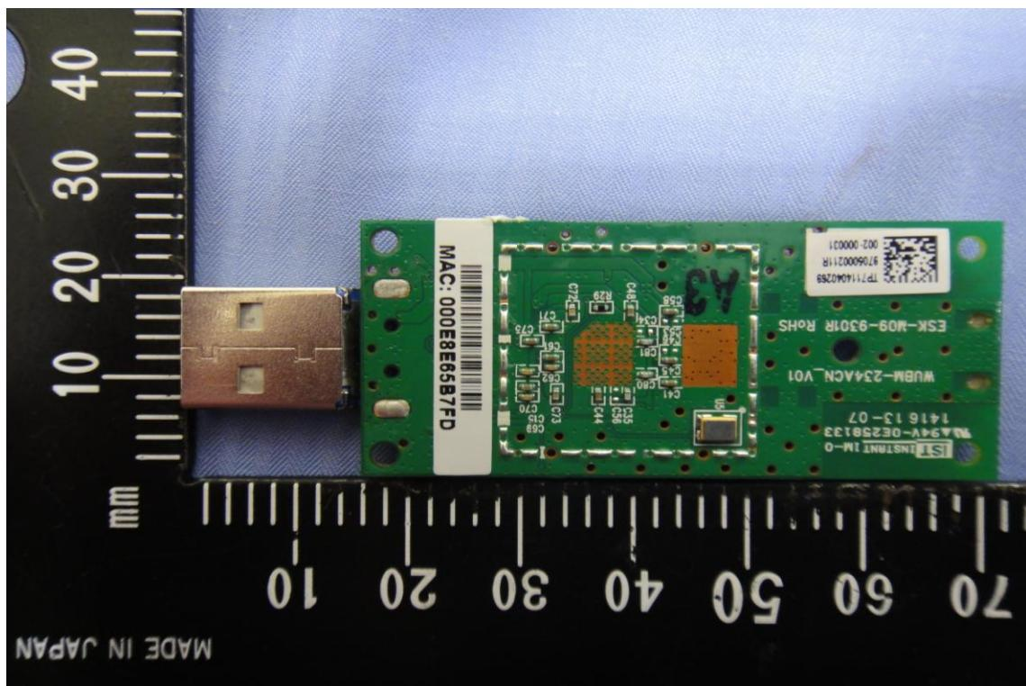
**For USB 3.0 type A + dipole antenna**
