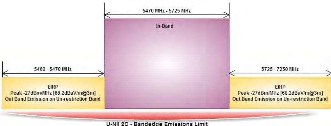
Refer as FCC KDB 789033 D02 v01, G)2)c)(i) specifying that if a non-restricted-band out-of-band emission satisfies both the average and peak limits of 15.209, it is not required to satisfy the -27 dBm or -17 dBm peak emission limit. Reason for change: to ensure that emission requirements in the non-restricted bands are not more stringent than those in the restricted bands.
