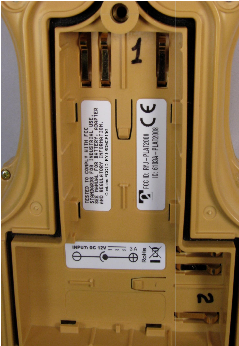
CLOSE-UP OF BATTERY COMPARTMENT SHOWING LABELS AND LABEL PLACEMENT
