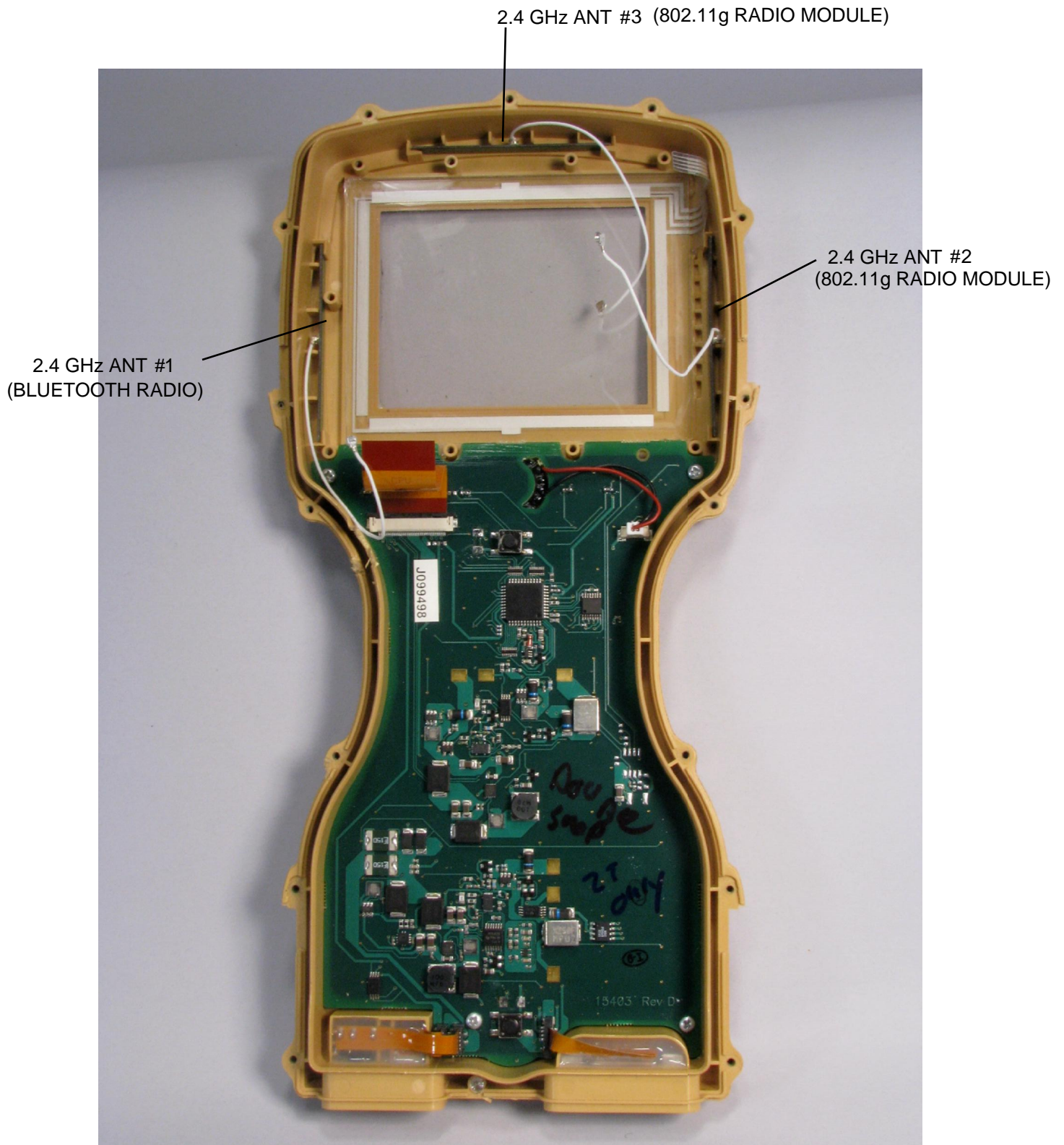
PHOTOGRAPH OF ANTENNAS IN PLAT2008 HOUSING
