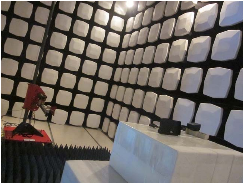
Measurement of Radiated Emission Test Set Up
