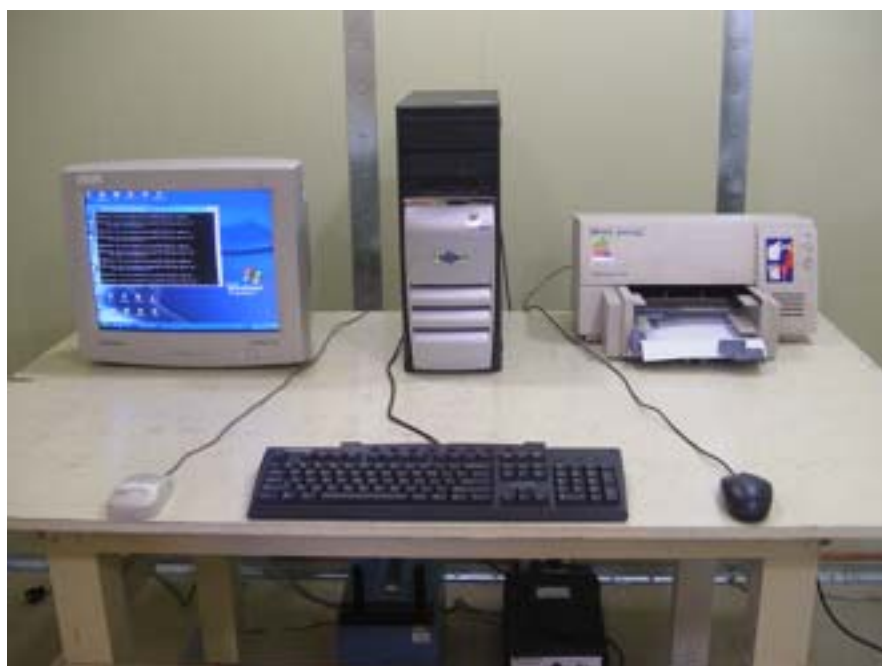
Photograph 2 : Setup for Conducted Emissions
