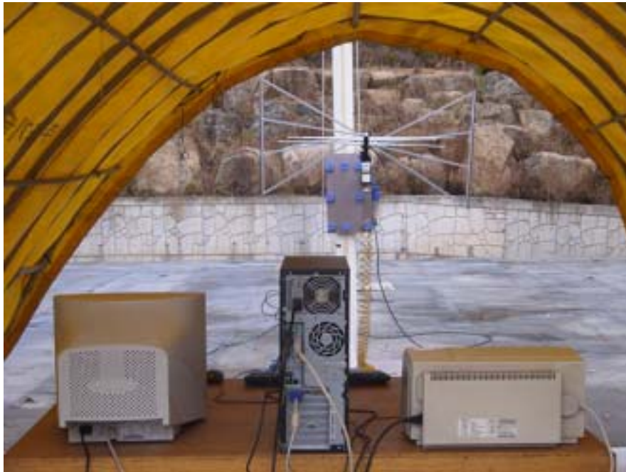
Photograph 1 : Setup for radiated Emissions
