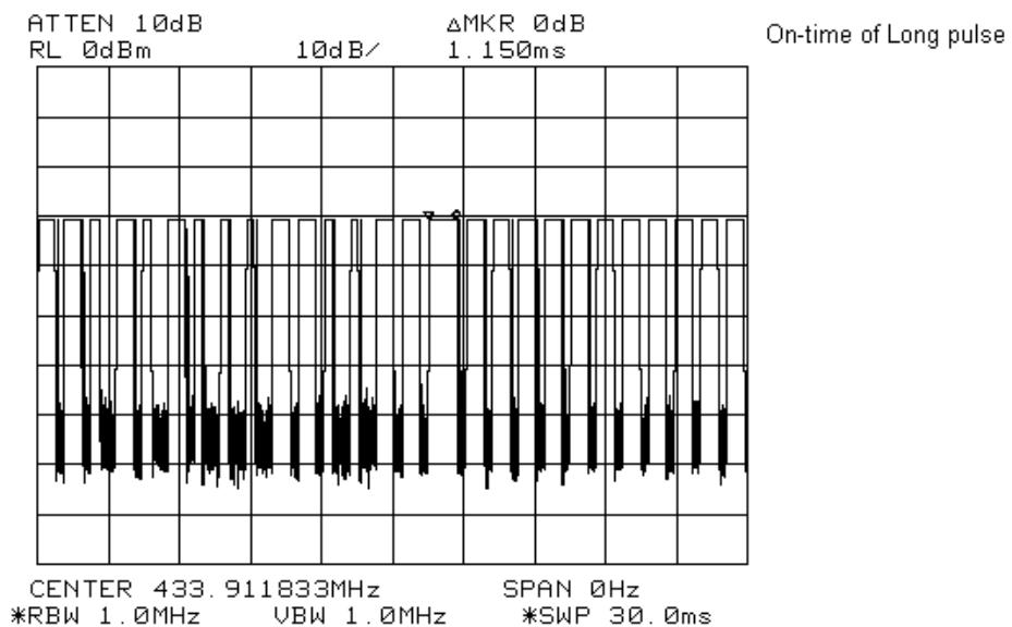
$$\text{Duty cycle} = 20\log((1.15\text{msec} \times 78)/100\text{msec}) = -0.9\text{dB}$$
