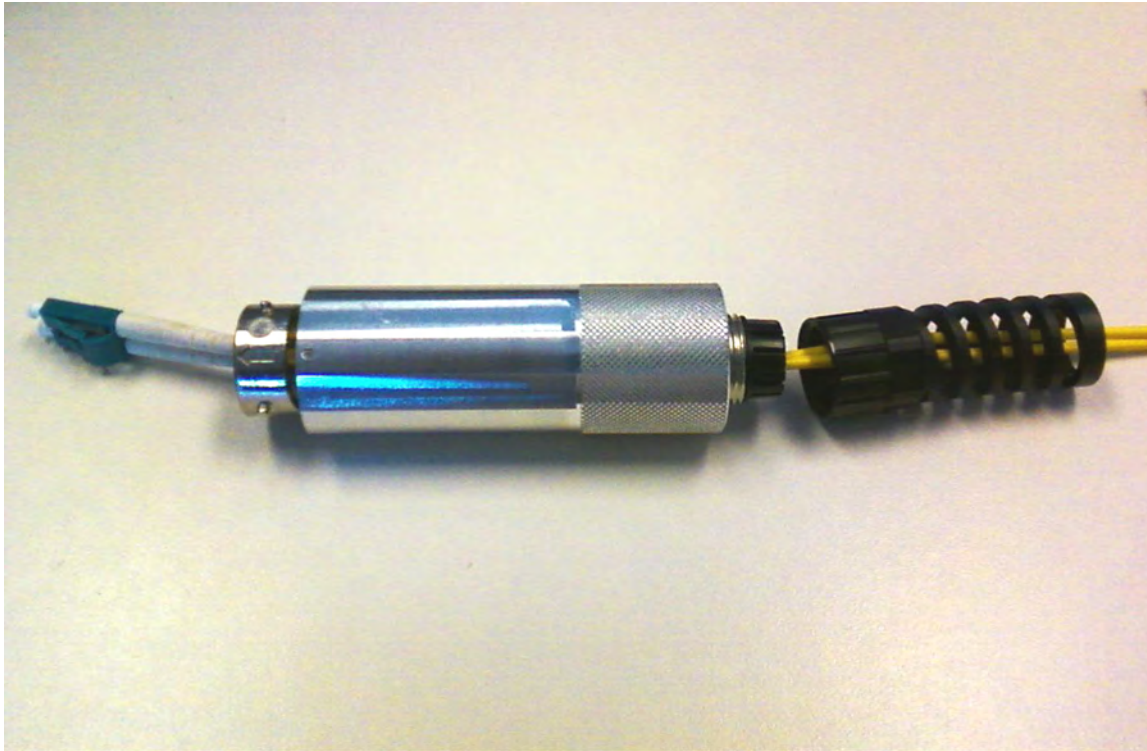
Figure 6-18 Inserting assemblies into the plug body
