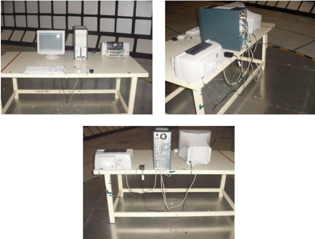
Figure 1 Test set up for radiated disturbance measurement
