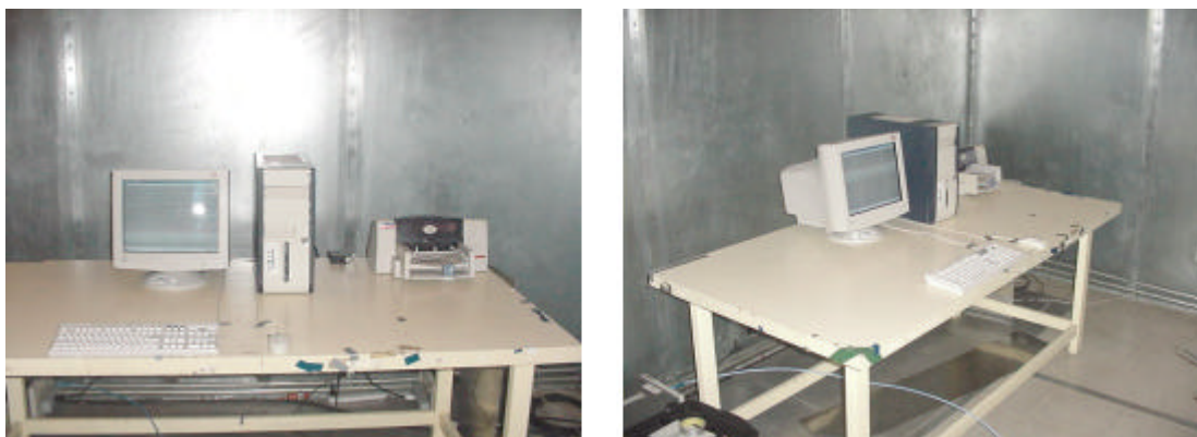
Figure 2 Test set up for conducted disturbance measurement
