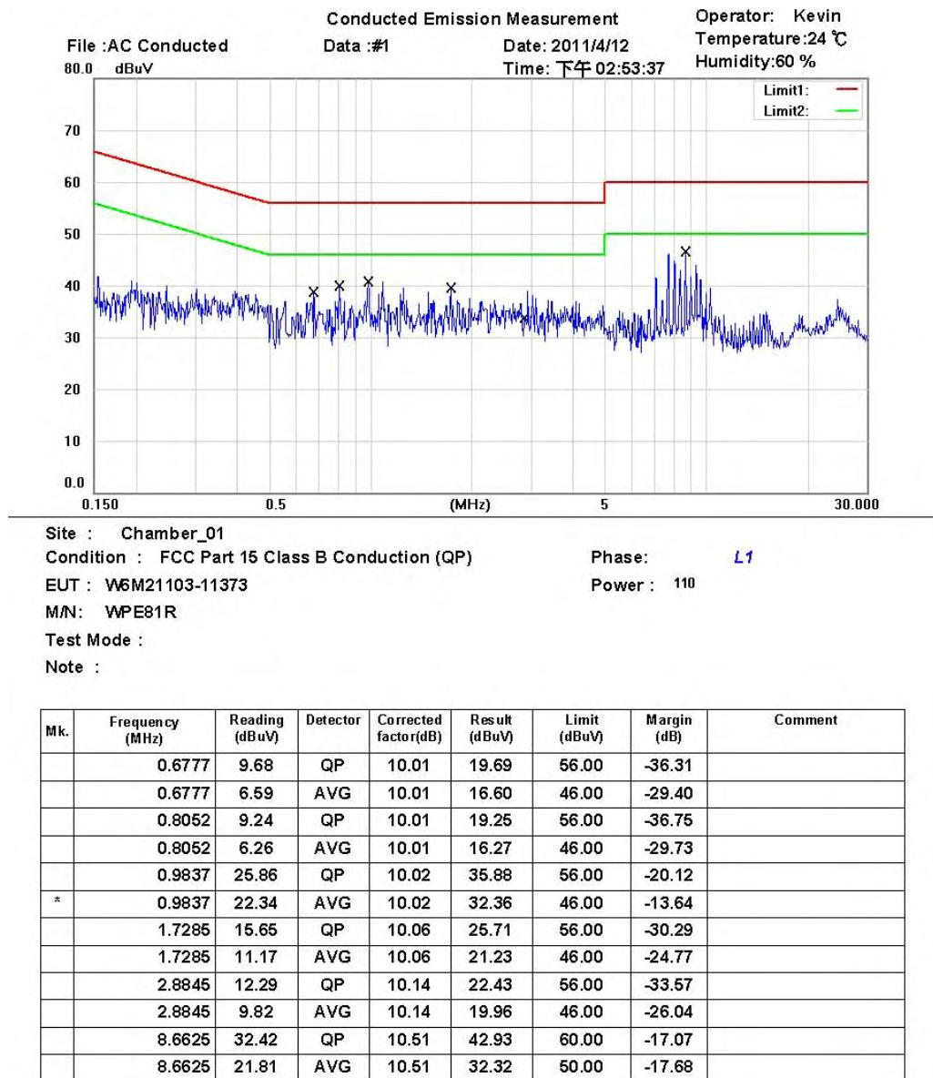
Note: 1. The formula of measured value as: Test Result = Reading + Correction Factor
