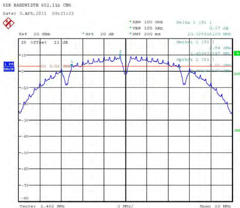
RF Spectrum Analysis Plot (Center: 2.462 GHz, Span: 20 MHz)
