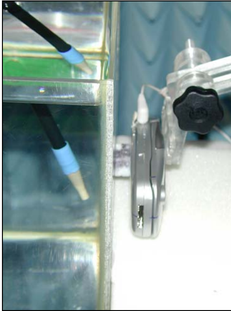
Figure 33. A Positional photograph of the MX-C110 Handset Fitted with Normal Battery positioned Rear Facing 10mm from the Flat Phantom
