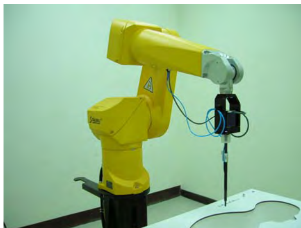
Fig. 5.2 Probe setup on robot
