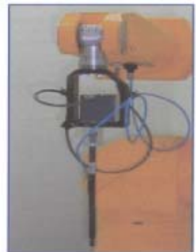
Figure4. ET3DV6 E-field probe
