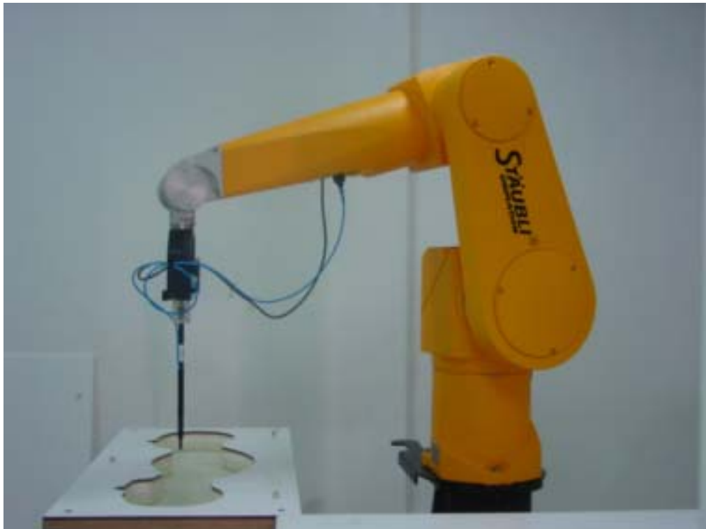
Picture 1 Specific Absorption Rate Test Layout
