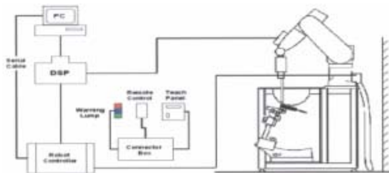
Figure2. SAR Lab Test Measurement Set-up
