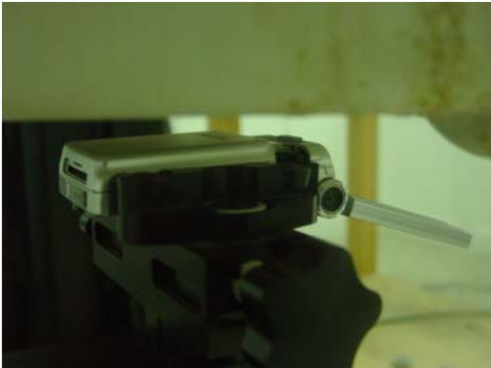
Picture 6 Flat Phantom -- Body-worn Position (towards ground, the distance from handset to the bottom of the Phantom is 1.5cm)
