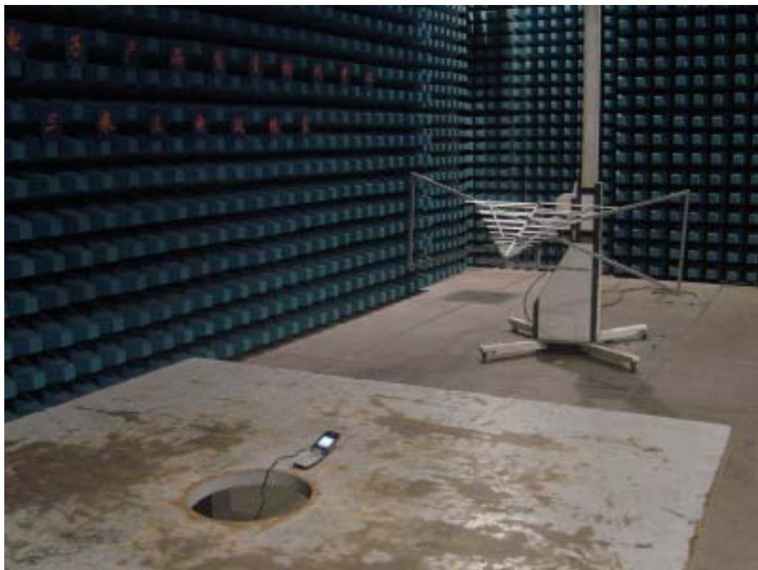
**4. Radiated Emission Test, USB Mode**
