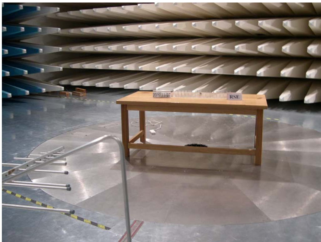
Pic C.2 Radiated Spurious Emission
