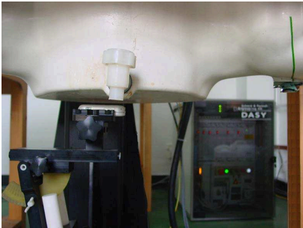
Picture B15: GPRS Body-worn Position with Bluetooth transmitter-flip closed (towards ground, the distance from handset to the bottom of the Phantom is 1.5cm)
