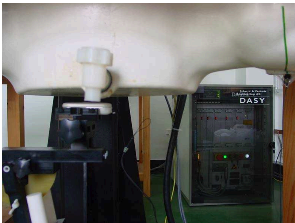
Picture B10: Body-worn Position with Flip Closed and Headset (toward phantom, the distance from handset to the bottom of the Phantom is 1.5cm)
