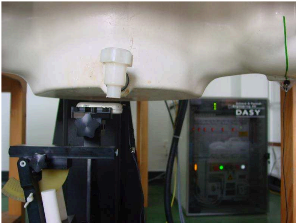
Picture B11: Body-worn Position with Flip Closed and Headset (toward ground, the distance from handset to the bottom of the Phantom is 1.5cm)
