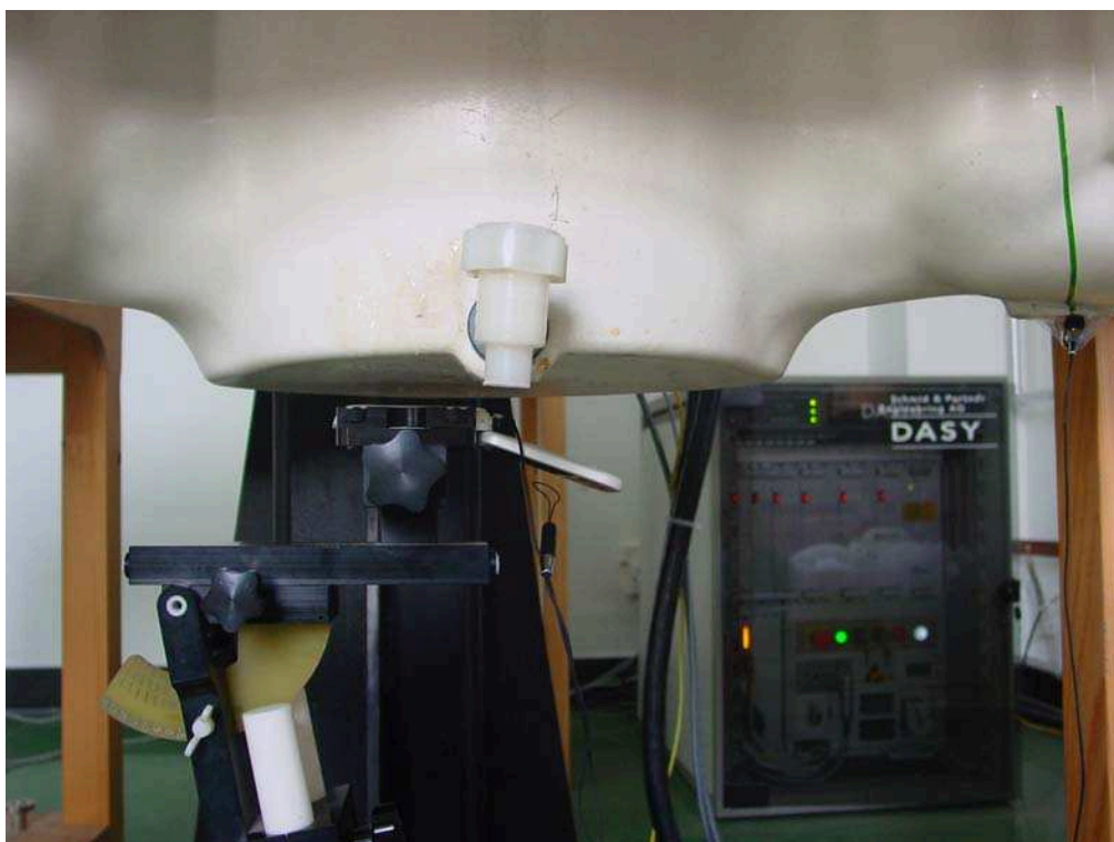
Picture B9: Body-worn Position with Flip Open and Headset (toward ground, the distance from handset to the bottom of the Phantom is 1.5cm)
