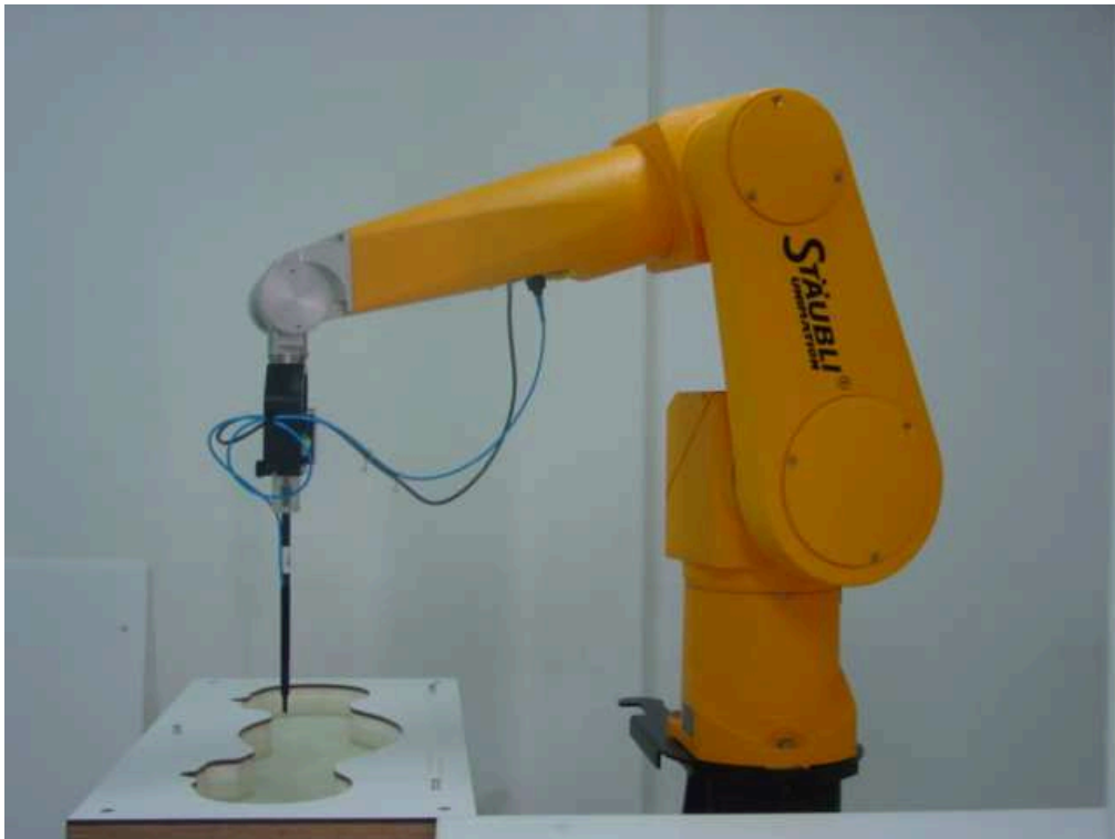
Picture B1: Specific Absorption Rate Test Layout
