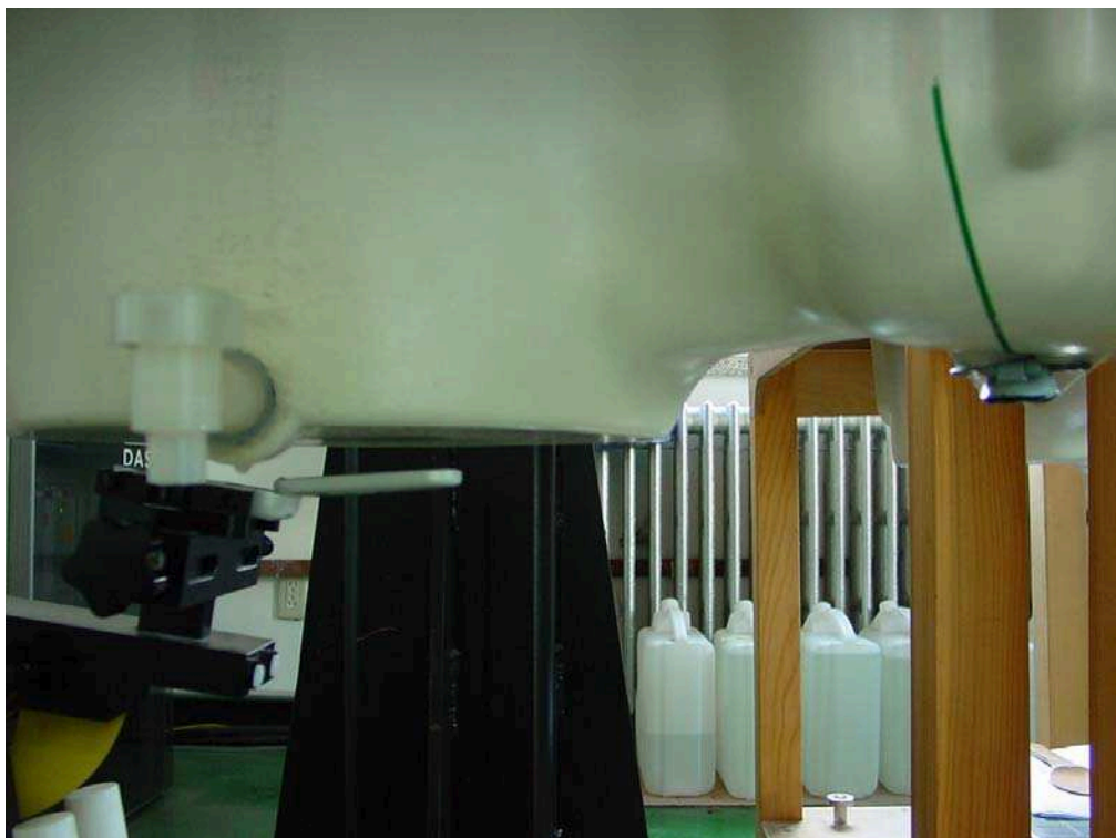
Picture B14: GPRS Body-worn Position with Bluetooth transmitter-flip open (towards phantom, the distance from handset to the bottom of the Phantom is 1.5cm)
