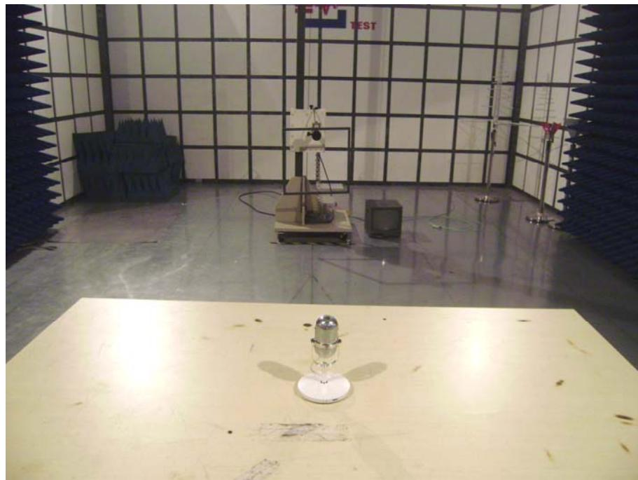
**Spurious Radiation Test Setup (30MHz to 1GHz)**
