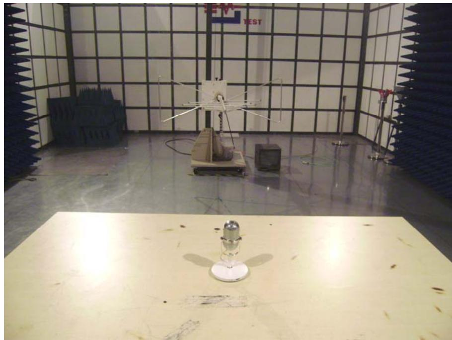
**Spurious Radiation Test Setup (Above 1GHz)**
