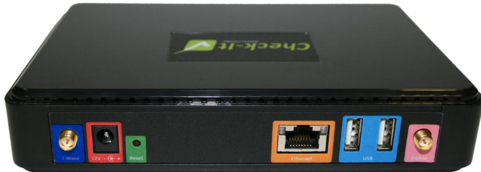
Figure 1: From left to right: Z-Wave™ antenna connector (dark blue), power connector (red), reset button (green), Ethernet jack (orange), USB ports (blue), and ZigBee™ antenna connector (pink).
