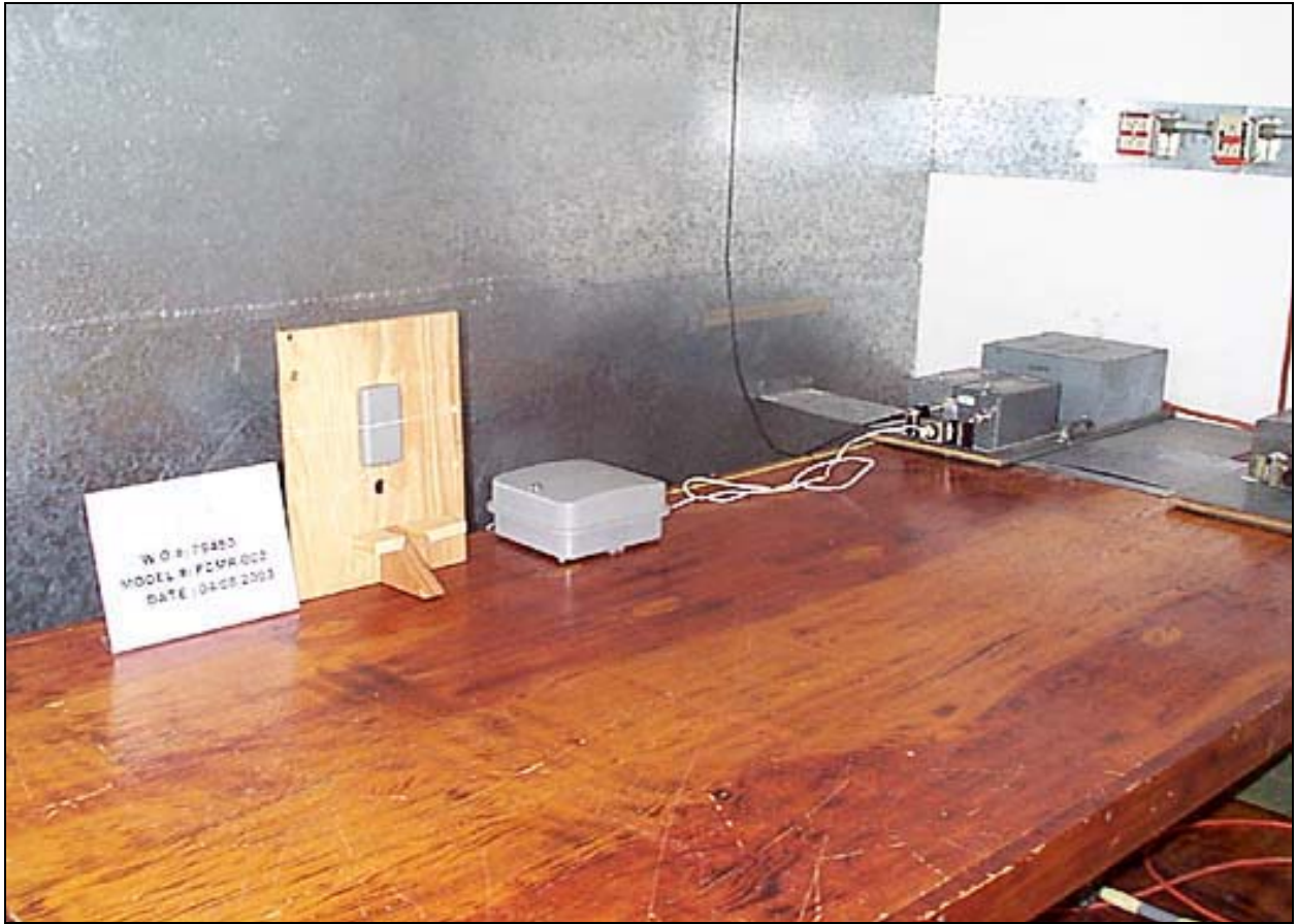
Test Setup Mains Conducted Emissions - Front View
