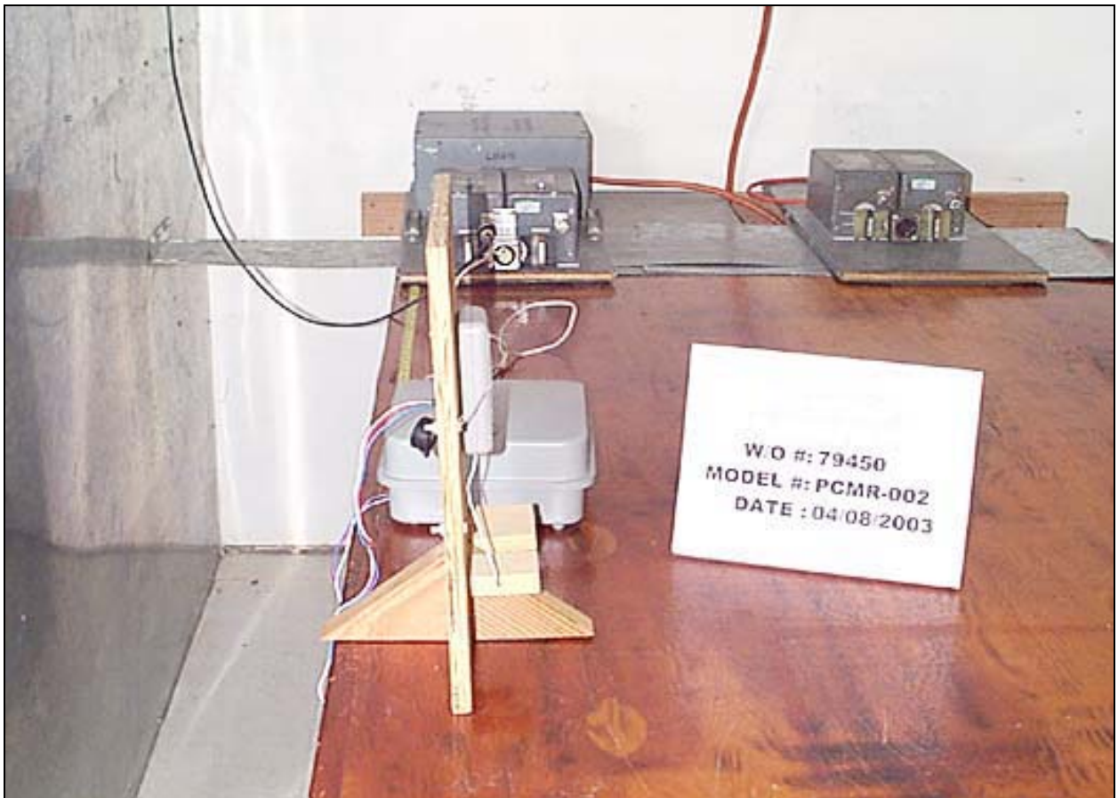
Test Setup Mains Conducted Emissions - Side View
