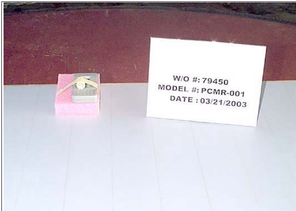
Test Setup Radiated Emissions - Y Axis
