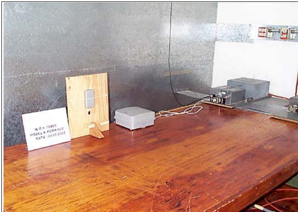
Test Setup Mains Conducted Emissions - Front View
