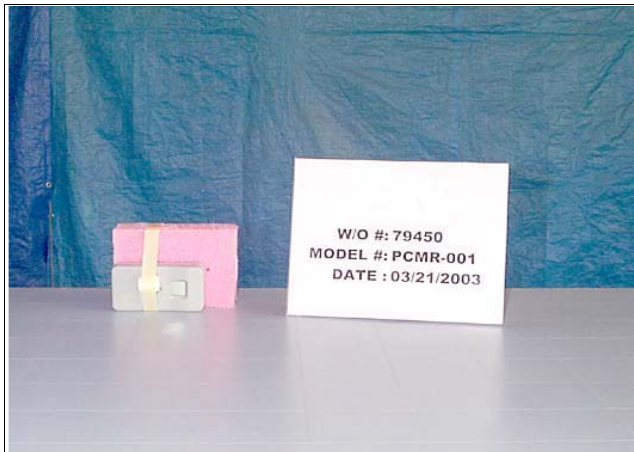
Test Setup Radiated Emissions - Z Axis
