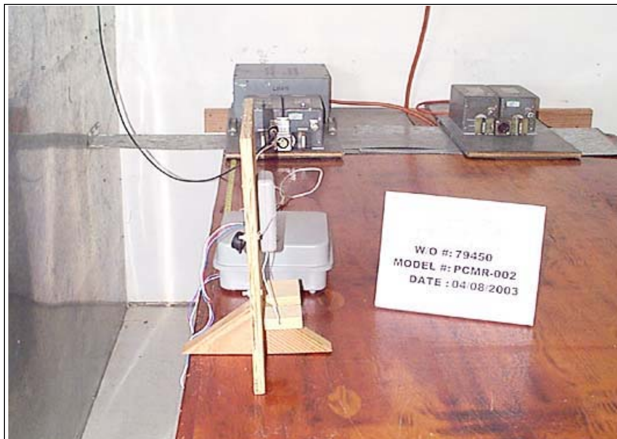
Test Setup Mains Conducted Emissions - Side View
