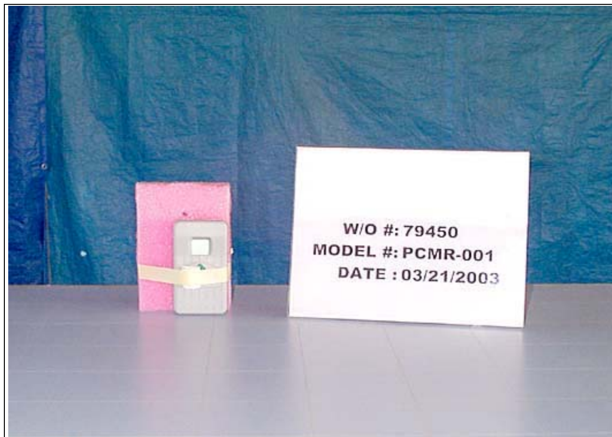
Test Setup Radiated Emissions - X Axis
