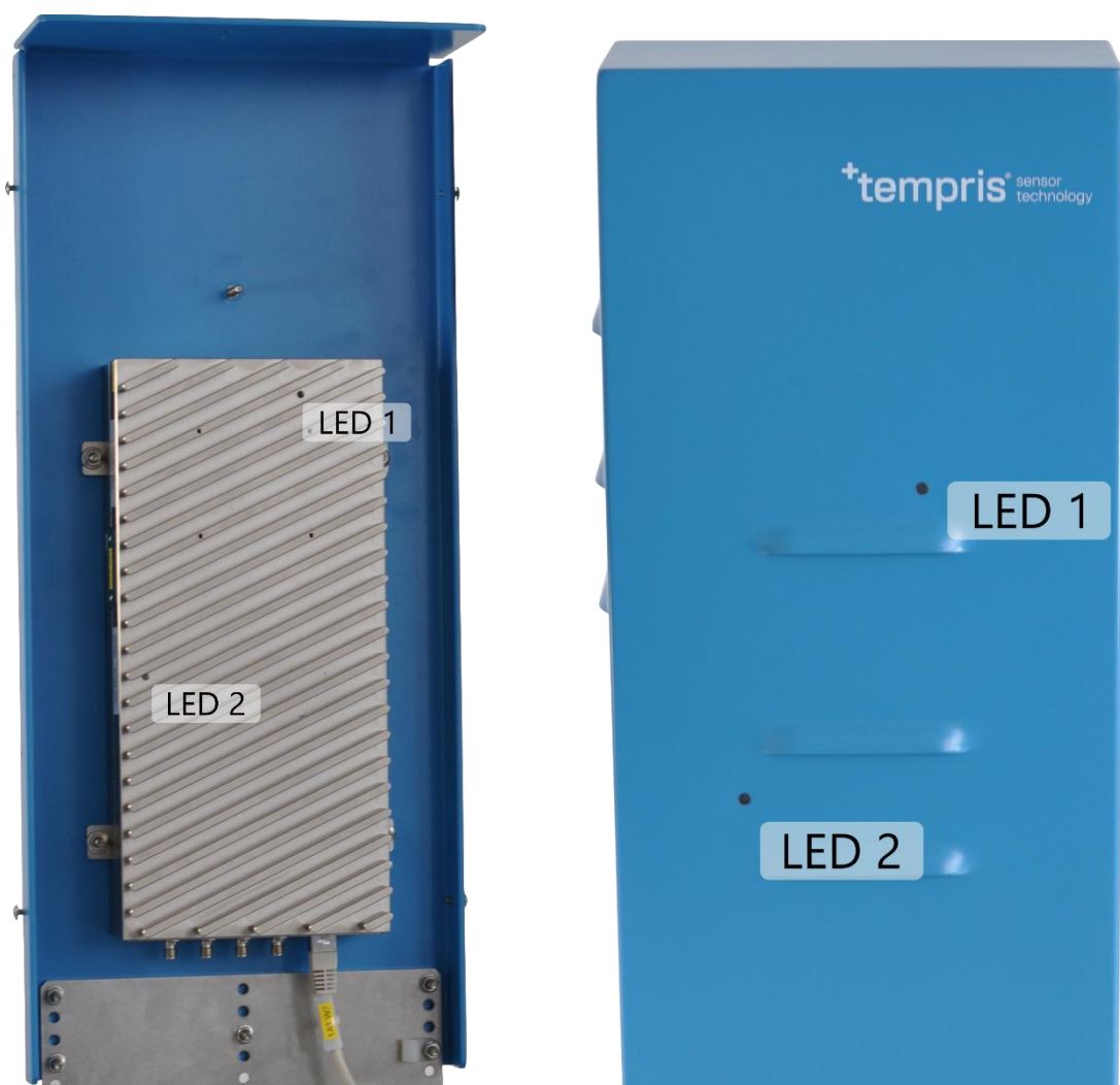
Figure 3-4: TIRU3 – Status LED 1 and 2 with opened and closed cover
