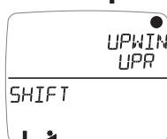
Sets the autoleg page to be displayed while the apparent wind angle is between head to wind and 90 degrees. The default is **Wind Shift**. Pages can be selected from any currently unhidden page.
