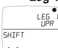
Sets the autoleg page to be displayed while the apparent wind angle is between head to wind and the leg1-2 changeover angle. The default is **Wind Shift**. Pages can be selected from any currently unhidden page.
