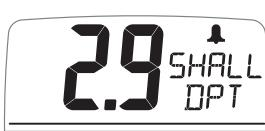
The water depth has fallen below the preset alarm level.
