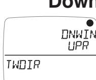
Sets the autoleg page to be displayed while the apparent wind angle is between 90 and 180 degrees. The default is **True Wind Direction**. Pages can be selected from any currently unhidden page.
