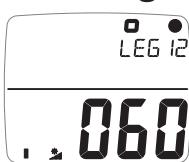
The angle at which the auto leg page switches from the Leg 1 page to the Leg 2 page. The default is **60 degrees**.
