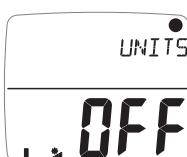
Configures the display to show the units of displayed values. By default this is set to **OFF** and no units are displayed.
