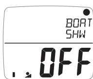
Allows the display to show information when NOT installed as part of a Micronet system for demonstration purposes only. Displays will return to **default OFF** on power down.
