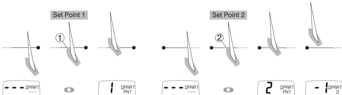
**Note:** The line for Depart calculations is between the positions you set. Set your points as close to the ends of the actual start line as possible.
