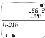
Sets the autoleg page to be displayed while the apparent wind angle is between the leg 1-2 changeover angle and the leg 2-3 changeover angle. The default is **True Wind Direction**. Pages can be selected from any currently unhidden page.
