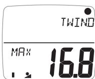
Resets the Dual Maximum True Wind Speed memory; resets to the current true wind speed.
