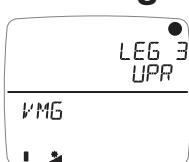
Sets the autoleg page to be displayed while the apparent wind angle is between the leg 2-3 changeover angle and 180 degrees. The default is **VMG to Windward**. Pages can be selected from any currently unhidden page.
