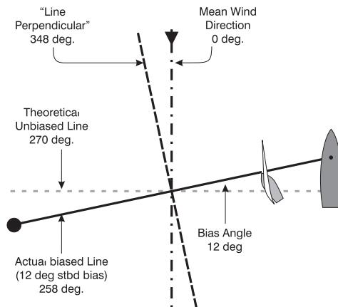
Your Dual Maxi Display can calculate and display the Line Bias angle and the favoured end of the line.
