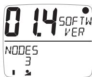
Displays the software version, battery level and charge rate to assist in troubleshooting and fault finding.
