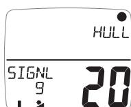
Shows the software version (large digits), signal strength and battery condition (level and charge rate) of the Hull Transmitter to assist in trouble shooting and fault finding
