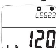
The angle at which the auto leg page switches from the Leg 2 page to the Leg 3 page. The default is **120 degrees**.
