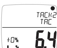
A value that corrects the speed displayed when the boat is on starboard tack, to take account of inherent differences of the measured speed on opposite tacks, e.g caused by off-centre installation of the transducer.
