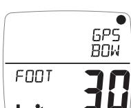
Sets the distance in feet of the GPS antenna from the bow of the boat. The default is **30 Feet**.
