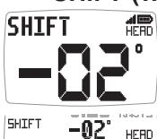
Indicates changes in the wind against a compass heading. Spotting these wind changes is the key to fast sailing upwind.
