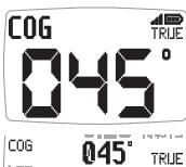
The vessel's course over the ground as calculated by the GPS Antenna or a GPS receiver.
