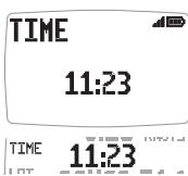
Current time as received from the GPS Antenna, corrected to local time if an offset has been added. See page 28 S37 to set an offset.
