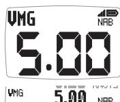
The vessel's speed directly towards the active Waypoint. This value is calculated by a GPS receiver or plotter.
