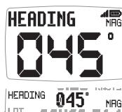
Current magnetic compass heading of the vessel as measured by the Compass Transducer.
