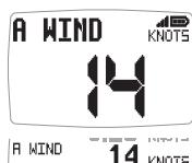
The apparent wind speed with respect to the vessel as measured by the Wind Transmitter, displayed in the currently selected wind units. See page 23 S11 to select wind units.
