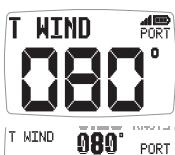
The true wind angle with respect to the vessel, calculated by the display taking into account the vessels speed through the water. Apparent Wind Speed, Angle and Boat Speed must be available for this calculation.
