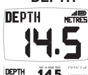
The actual depth beneath the vessel as measured by the Depth Transducer.
