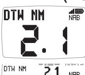
Distance to active Waypoint. The active waypoint being the one to which the GPS is currently navigating as defined by a GPS receiver or plotter.
