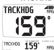
Magnetic compass heading that the vessel will follow should it tack through the wind, calculated by the display. Apparent Wind Angle and Magnetic Heading must be available for this calculation to be made.
