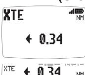
The distance away from the direct track to the (active) waypoint as defined by a GPS receiver or plotter.
