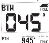
Bearing to (active) waypoint. The active waypoint being the one to which the GPS is currently navigating as defined by a GPS receiver or plotter.
