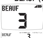
The actual wind speed over the water displayed using the Beaufort scale, calculated by the display taking into account the vessels speed through the water and compass heading. Apparent Wind Speed, Angle and Compass Heading must be available for this calculation.
