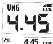
The vessel's calculated Speed Directly Upwind. This value is calculated by the display from the Boat Speed and True Wind Angle.
