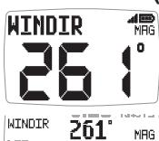
The true wind direction over the water, calculated by the display taking into account the vessels speed through the water and compass heading. Apparent Wind Speed, Angle and Compass Heading must be available for this calculation.
