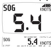
The vessel's speed over the ground as calculated by the GPS Antenna or a GPS receiver.
