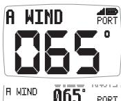
The apparent wind angle with respect to the vessel as measured by the Wind Transmitter.
