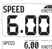
The vessel's actual speed through the water as measured by the Speed Transducer, displayed in the currently selected speed units. See page 22 S9 to set units.
