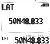
The vessel's current latitude as calculated by the GPS Antenna or a GPS receiver.
