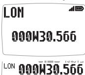
The vessel's current longitude as calculated by the GPS Antenna or a GPS receiver.
