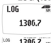
The total distance travelled by the vessel since installation of the display or since a Factory Reset. See page 29 S40 to reset.
