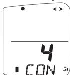
Adjusts the viewing angle of the LCD display to improve visibility under varied mounting possibilities.
