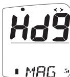
The system can be configured to show heading information in either **MAG (Magnetic)** or **TRU (True)** format. Magnetic Variation must be set to enable True display format (see section above). A True Heading is indicated by the TRUE icon in the upper pane; the absence of this icon indicates a Magnetic heading.
