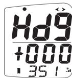
Aligns the displayed heading with the actual magnetic heading of the boat (see page 17 for the calibration process).
