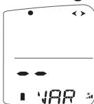
Allows manual entry of local magnetic variation. A value between W90 degrees and E90 degrees.
