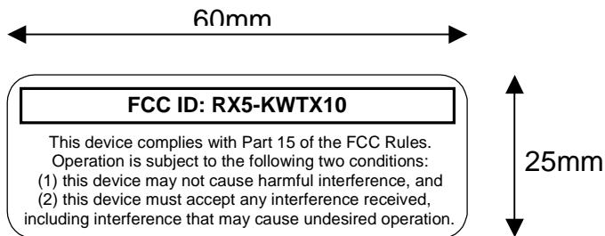
The label is to be printed white on black, fixed onto the left side of the transmitter unit.
