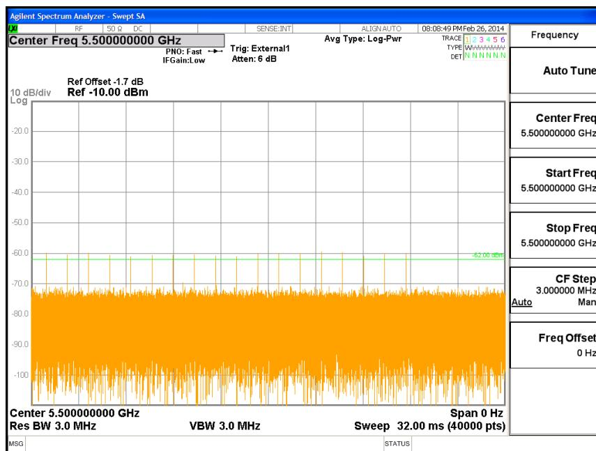
**<40MHz / 5510 MHz> Radar Type 1****Radar / DFS detection threshold level and the burst of pulses on the Channel frequency**
