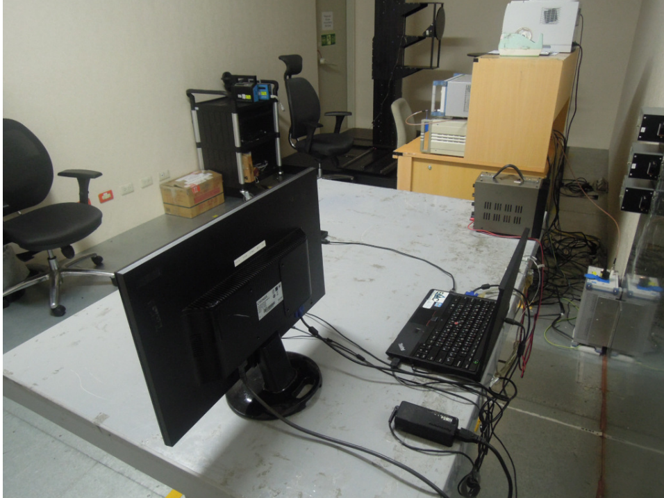
Photograph 7: Set-up for Mains Conducted testing (Back View)
