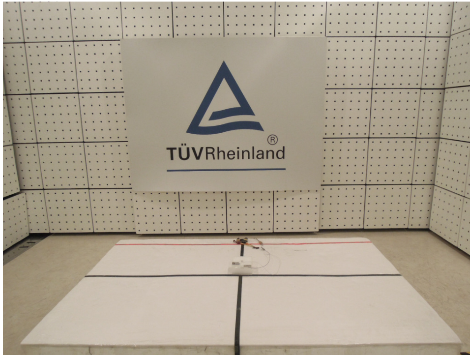
Photograph 1: Set-up for Spurious Emissions (Front View)
