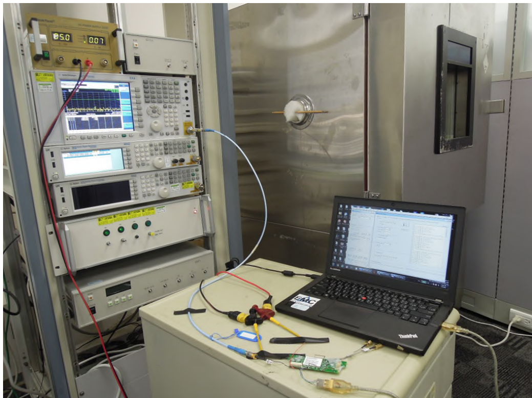
Photograph 4: Set-up for Conducted testing
