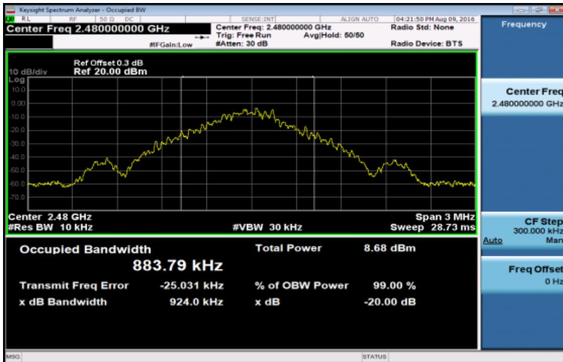
20dB Band Width Test Data CH-Low ( $\pi/4$ -DQPSK mode)
