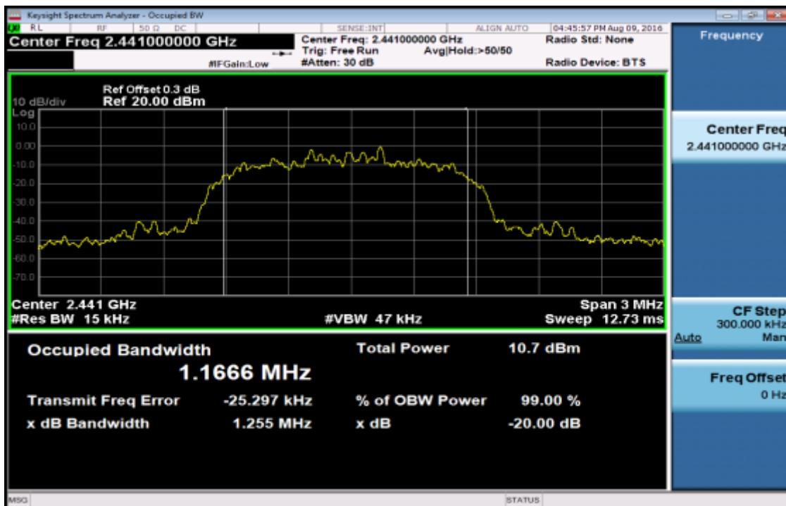
20dB Band Width Test Data CH-High ( $\pi/4$ -DQPSK mode)
