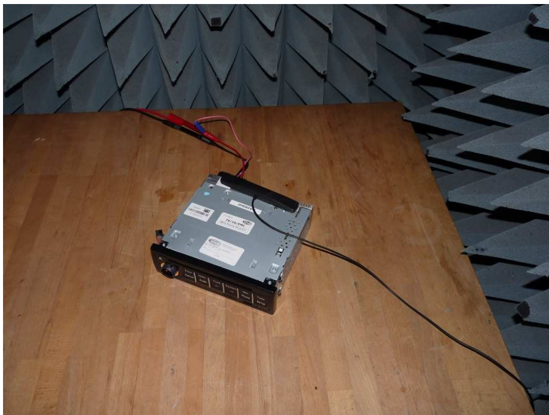
Photo 1: Setup for radiated measurements below 30 MHz
