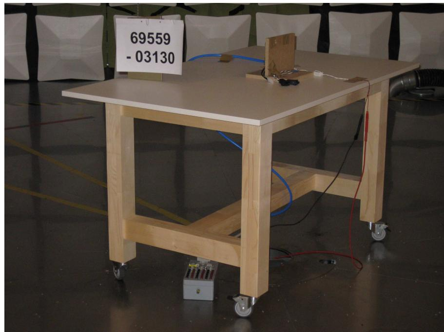
**Test setup for radiated emission measurement
