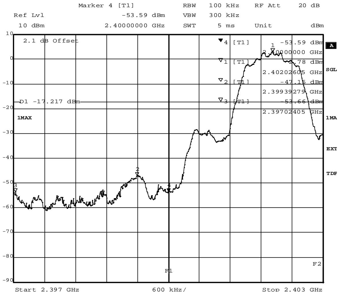
(determination of reference value for spurious emissions measurement)
