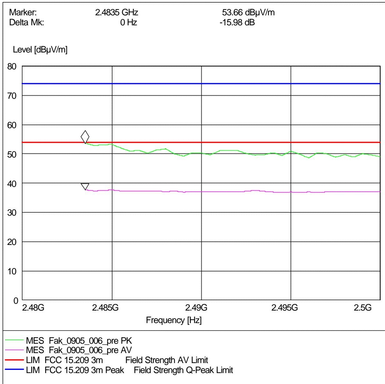
Radiated measurement (higher band edge)
