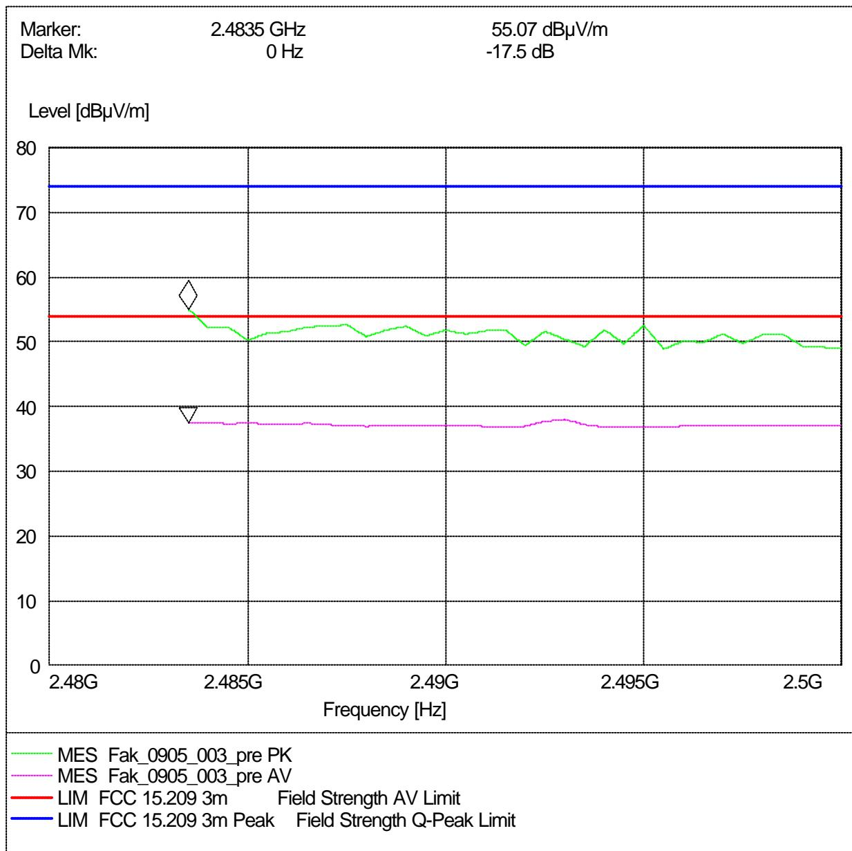
Radiated measurement (higher band edge)
