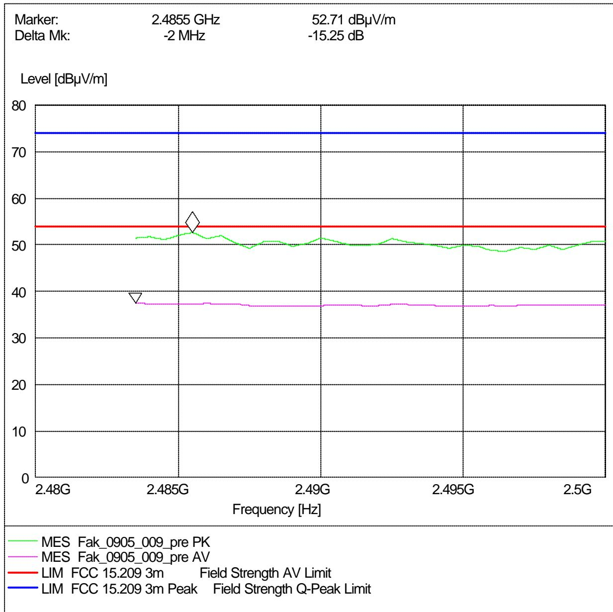
Radiated measurement (higher band edge)
