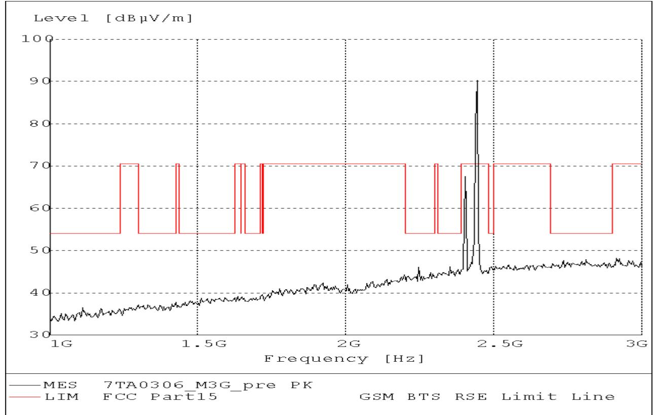
Note: the peak above the limit is carrier power
