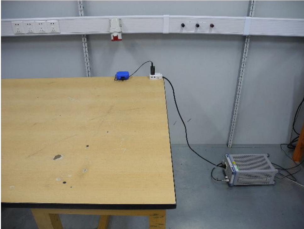
Photograph 6: Set-up for Radiated Emissions, below 1GHz
