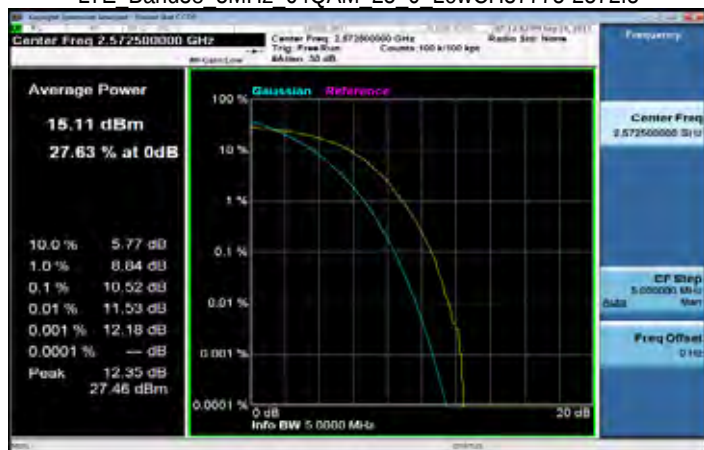
LTE Band38 5MHz 64QAM 25 0 LowCH37775-2572.5
